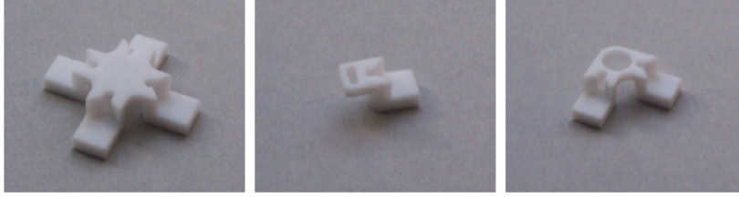
Figure 5.5: The three different types of Teflon block used to hold the crystals in the copper frames.
